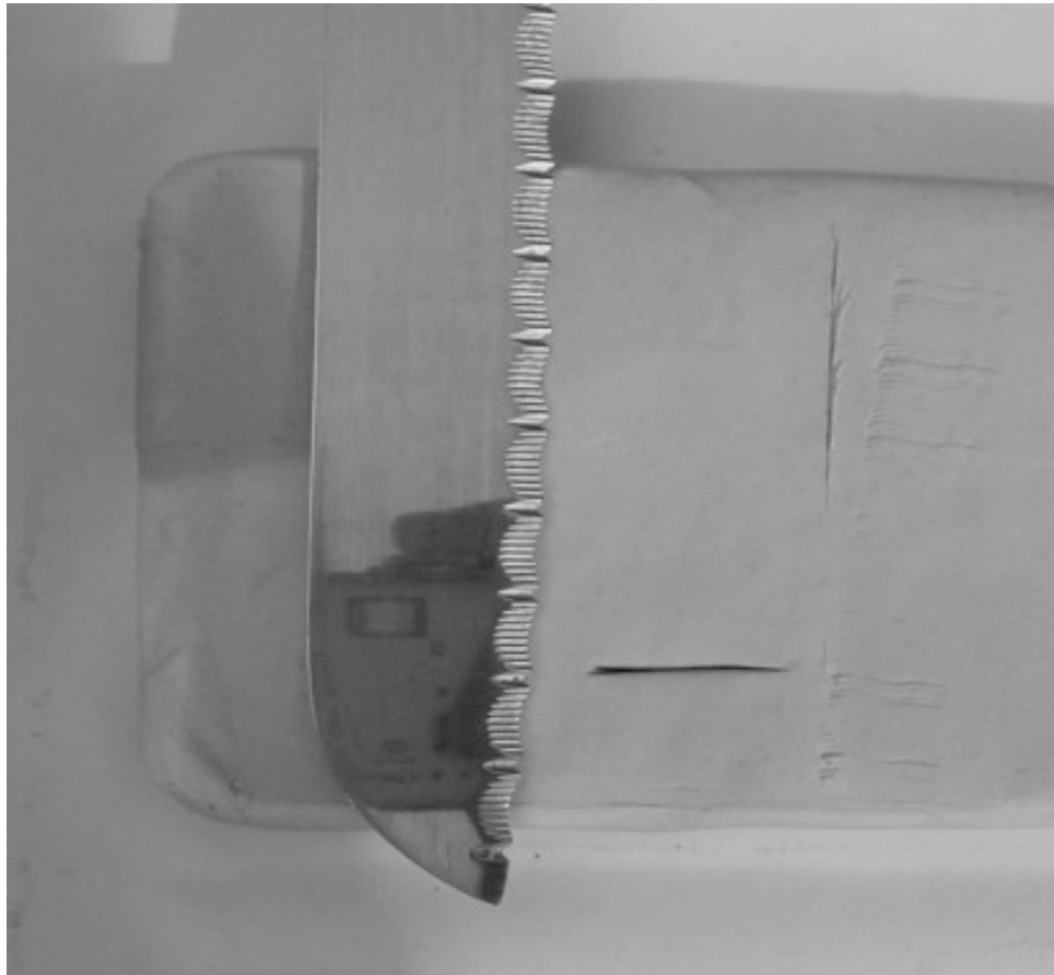
Fig. 180. This image is of a serrated kitchen knife (note the impression of the blade penetration into modeling clay and serration marks from 'dragging' the knife across the clay surface. ( www.forensicmed.co.uk )
